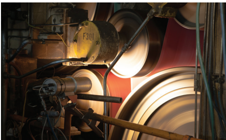
PulpInspector cameras can be synchronized with other monitoring and inspection cameras on the machine to identify the origin of defects in the sheet.
