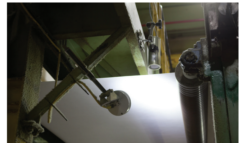
PulpInspector cameras can be synchronized with other monitoring and inspection cameras on the machine to identify the origin of defects in the sheet.
