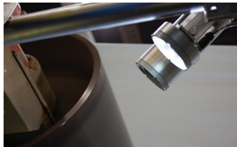
PulpInspector cameras can be synchronized with other monitoring and inspection cameras on the machine to identify the origin of defects in the sheet.
