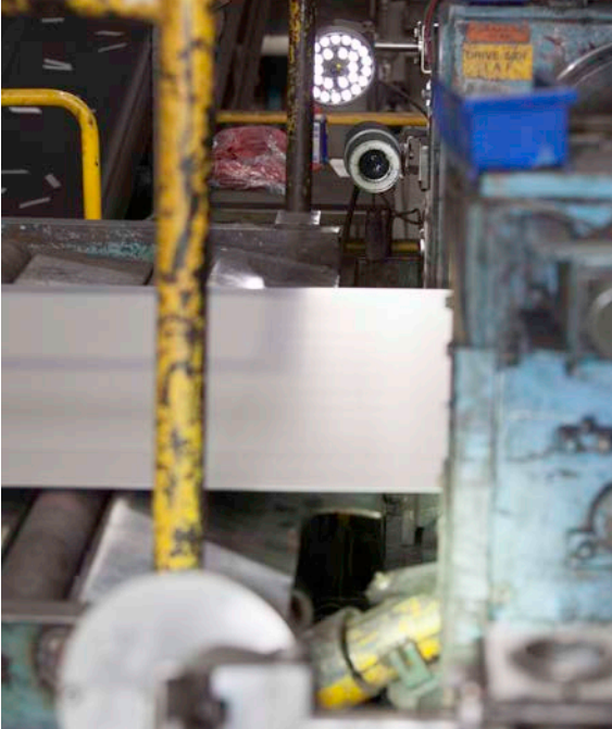
Opposing cameras and lights are synchronized to avoid interfering with each others' imaging.
