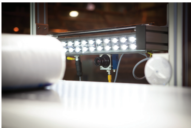
Lighting is application matched. Here a light highlights the top edge of a tissue package where the plastic wrap is folded and sealed.
